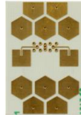
Full integrated radar front end, 24GHz. Pricing << 5 Euro in large qts
